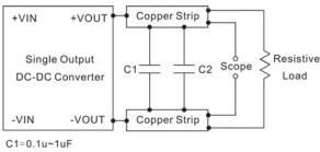
Use a Cout ceramic capacitor. Please refer to capacitor value of every series. Scope measurement should be made by using a BNC socket, measurement bandwidth is 0-20 MHz. Position the load between 50 mm and 75 mm from the DC-DC Converter.
