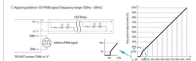
Duty cycle of additive 10V PWM signal dimming input
