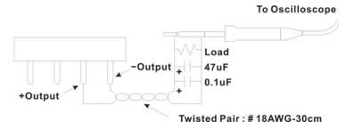
47uF and 0.1uF capacitor of proper polarity and voltage rating. The oscilloscope probe ground led should connect right to the ground ring of the probe and be as short as possible. The oscilloscope bandwidth should be at 20MHz and connected to AC ground.
