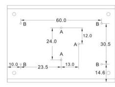
A= For fixture to chassis only A=M3x0.5P B=For fixture to pcb/chassis only B=M3x0.5P Torque:3±0.5 Kgf.cm
