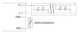
"DO NOT connect "DIM- to -V"
