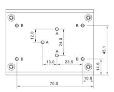
A= For fixture to chassis only A=M3x0.5P B=For fixture to pcb/chassis only B=M3x0.5P Torque:3±0.5 Kgf.cm
