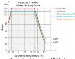
If input voltage is lower than 100VAC, please refer to the output derating V.S. input voltage curve for details
